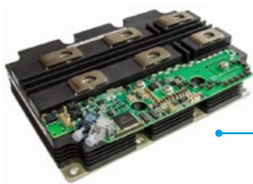
Latest generation of HV 6.5 kV IGBTs
