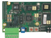
现场总线通信套件 Profibus DP → KFB-PD DeviceNet → KFB-DN Profibus DPV1 → KFB-PDPV1 DeviceNet Acyclic → KFB-DD 以太网/IP → KFB-ENIP
